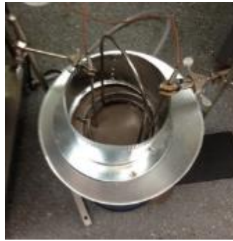
Figure 5.7 Modification to sand bath to limit spills
