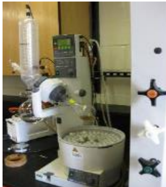
Figure C.2 Büchi R-205 rotary evaporator (Brinkmann Instruments, Inc., Westbury, NY, U.S.A)
