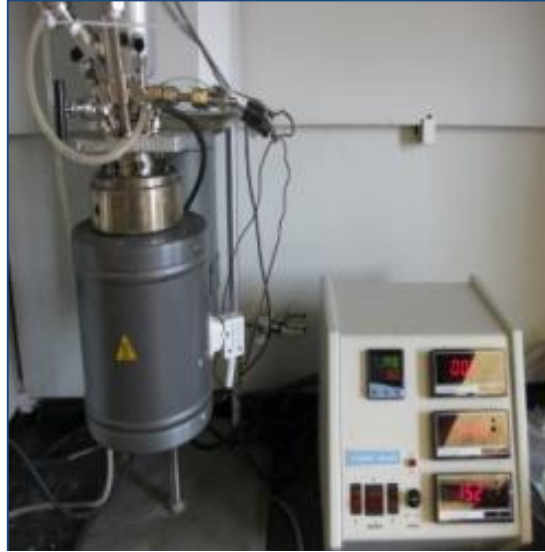
Figure 5.5 Four hundred and fifty milliliter (450-ml) Parr® reactor for the supercritical methanol transesterification of activated sewage sludge.
