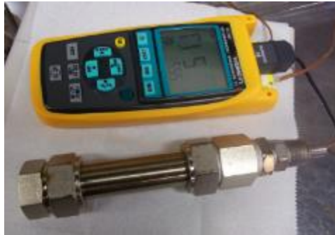
Figure C.4 Datalogger used to record internal probe and sand bath temperature changes
