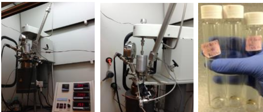
Figure 3.16 Final modification to 450-ml Parr® reactor used for final kinetic study in transesterification of soybean oil
