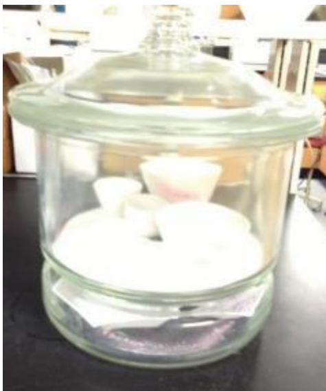
Figure C.5 Dessicator used for holding catalysts till use (Fisher Scientific, Pittsburgh, PA, USA)
