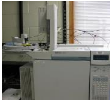
Figure 5.14 Agilent 6890 series GC system with DA Stabilwax column for quantifying FAMES and FFA Initial and final temperatures of 50 °C and 250 °C
