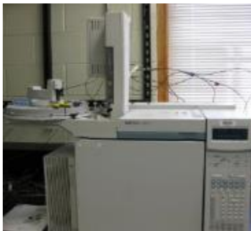
Figure 4.7 HP 6980 series GC system with DA Stabilwax column for quantifying FAMES and FFA Initial and final temperatures of 50 ^{\circ}\text{C} and 250 ^{\circ}\text{C}
