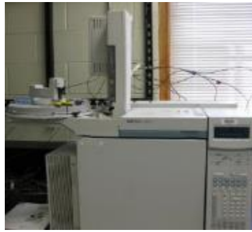
Figure 3.17 Agilent 6890 series GC system with DA Stabilwax column for quantifying FAMES and FFA Initial and final temperatures of 50 °C and 250 °C
