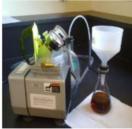
Figure 3.9 Gast Oil-less Vacuum pump set-up for catalyst filtration (Fisher Scientific, Pittsburgh, PA, USA)
