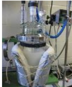
Figure 3.10 1000ml 3-necked reactor equipped with stirrer and temperature controller (Chemglass Inc., Vineland, NJ, USA)
