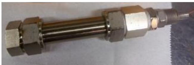
Figure 5.9 Temperature probe fitted to the reactor
