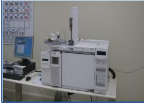
Figure 5.16 Agilent 5975 GCMS with Mass Selective Detector (MSD)
