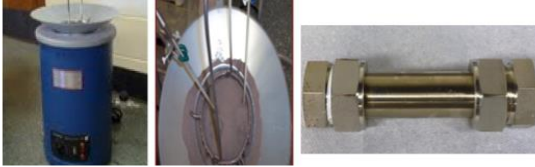
Figure 5.6 Fluidized sand bath and 46-ml reactor from Swagelok® tubing for the supercritical methanol transesterification of activated sewage sludge and Rhodotorula glutinis .
