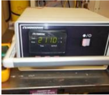
Figure C.3 Benchtop temperature controller for sand bath (Omega Engineering, Stamford, Connecticut, U.S.A.)
