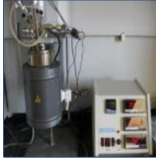
Figure 3.7 Parr 5522 - 450ml reactor (Parr Instrument Company, Moline, IL, U.S.A)
