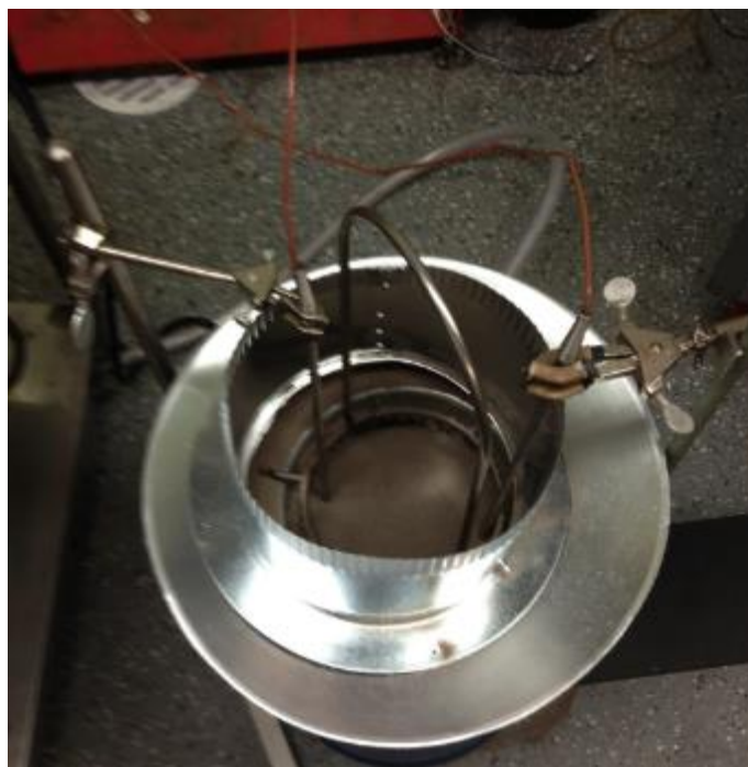
Figure 5.13 Modified fluidized sand bath with air duct restraining sand loss
