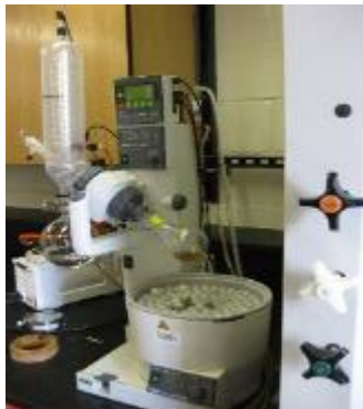
Figure 3.8 Büchi R-205 rotary evaporator (Brinkmann Instruments, Inc., Westbury, NY, U.S.A.)
